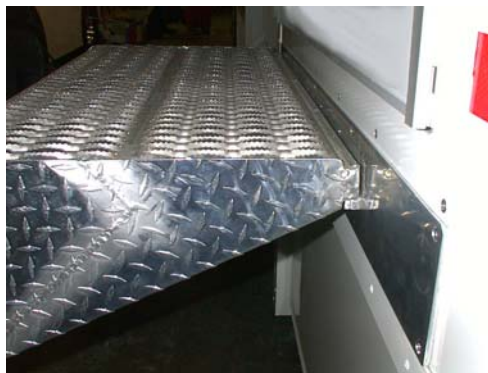
Figure 22: Stair Assembly (standard)
