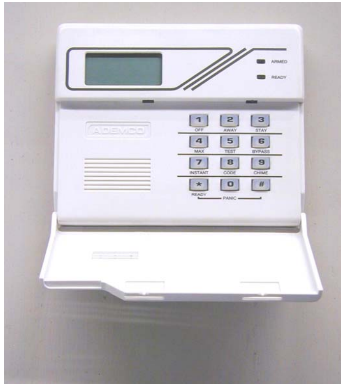
Figure 52: Intrusion Alarm Keypad
